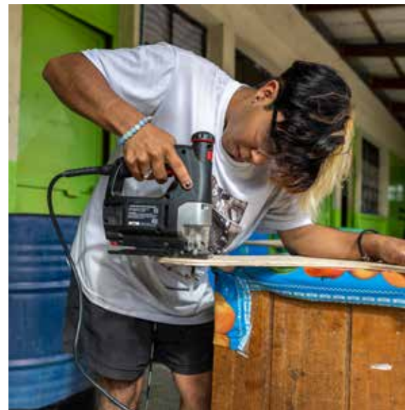
Julio Lopez cuts pieces of wood to replace the rotting parts of desks at the school.
